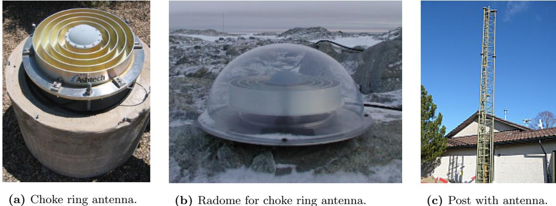
(a) Choke ring antenna. (b) Radome for choke ring antenna. (c) Post with antenna.
