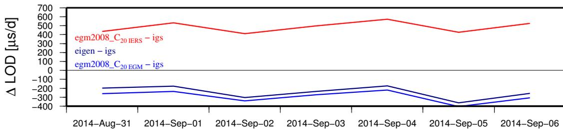
**Figure 3:** Differences in length of day (LOD) estimates with respect to IGS Final combined LOD product (igs) based on different internal GFZ solutions. eigen: *EIGEN\_GLO4C* gravity model, egm2008\_C<sub>20</sub>IERS: *EGM2008* gravity model but with supplemented IERS2010 C<sub>20</sub>-term (from Tab. 6.2 in [Petit and Luzum 2010](#)); egm2008\_C<sub>20</sub>EGM: *EGM2008* gravity model.
