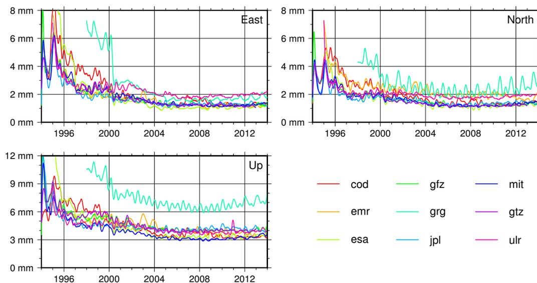
**Figure 5:** WRMS of AC station position residuals from preliminary combinations of the daily AC repro2 SINEX solutions. All time series were low-pass filtered with a 2.5 cycles per year cut-off frequency.
