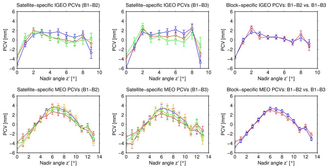
**Figure 2:** Satellite- and block-specific IGSO (top) and MEO (bottom) PCV estimates together with error bars representing the formal errors from the variance-covariance matrix. Results for IGSO-4/5 are not shown for reasons of clarity.
