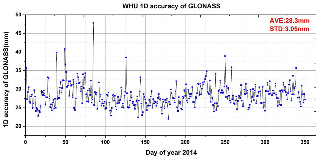
Figure 4: GLONASS orbit compared with IGL final solution.
