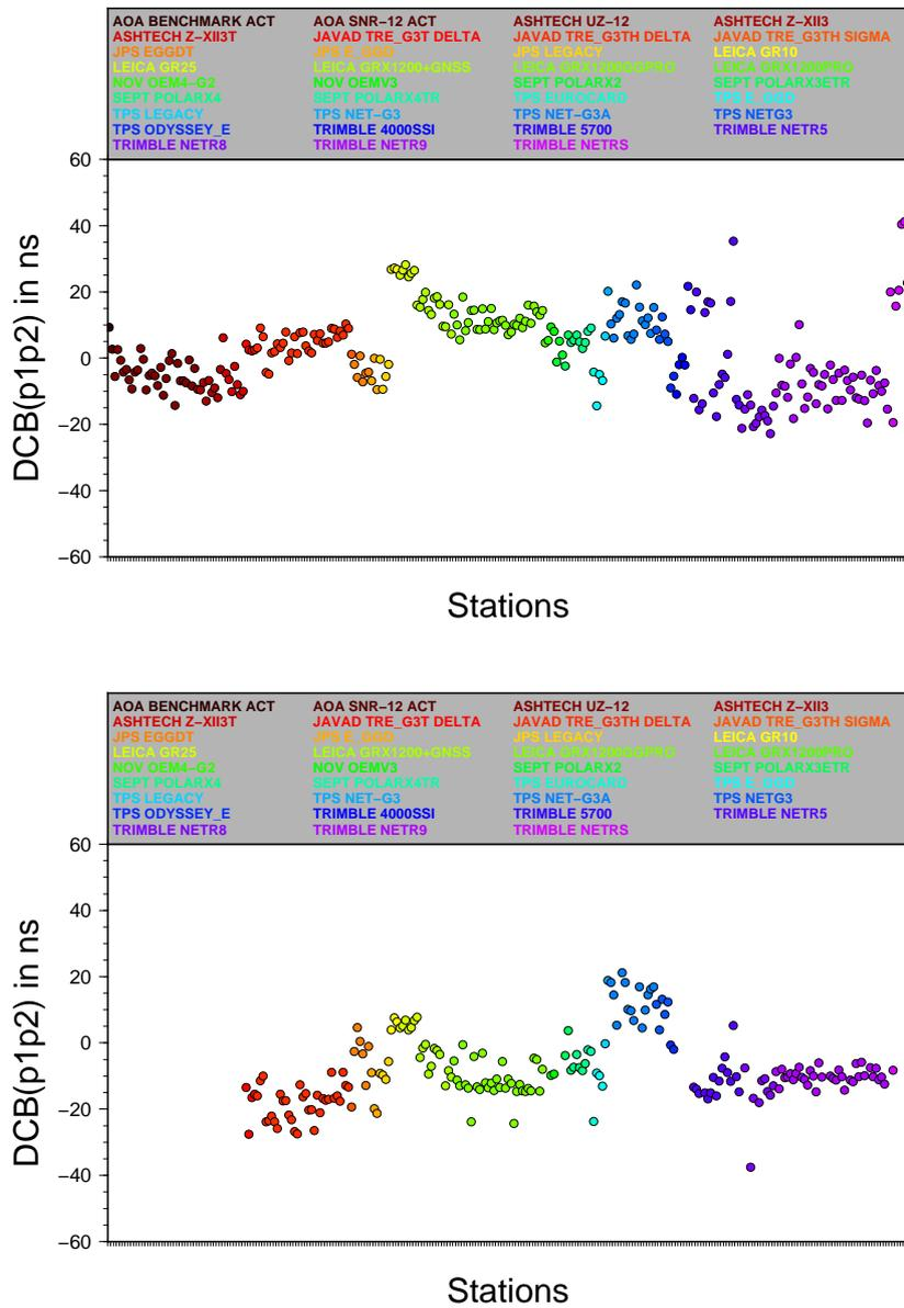
**Figure 3:** Monthly set of P1-P2 differential code biases for the GPS (top) and GLONASS (bottom) receiver components, for December 2014, computed at CODE.
