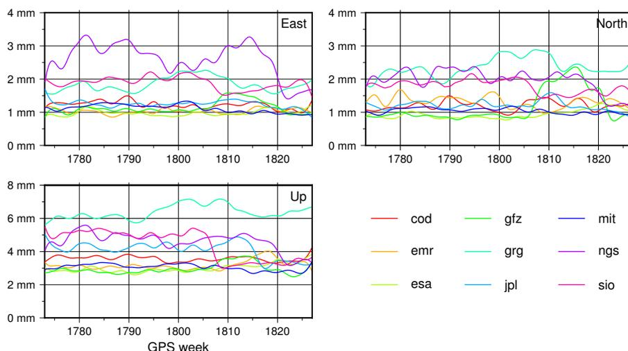
**Figure 1:** RMS of AC station position residuals from the 2014 daily IGS SINEX combinations. All time series were low-pass filtered with a 10 cycles per year cut-off frequency.
