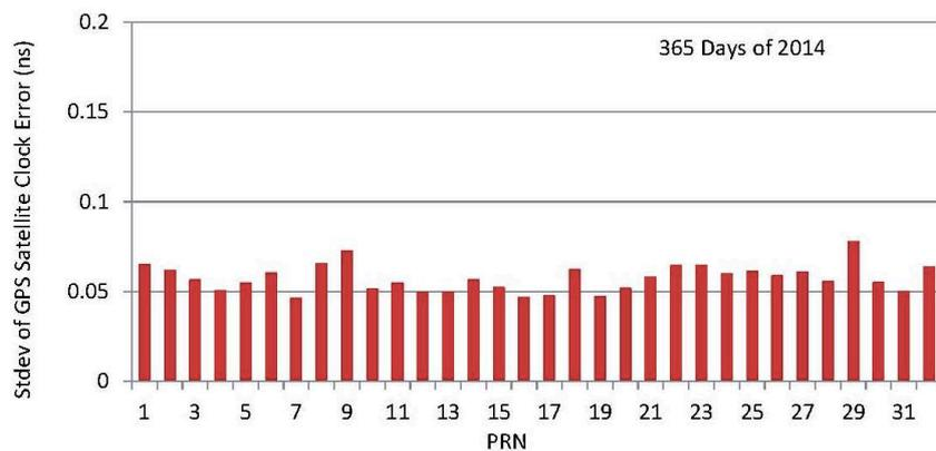
**Figure 10:** The STD of real time clock error of GPS satellites.
