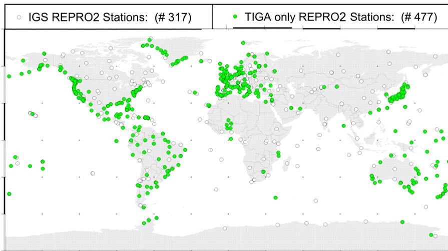
**Figure 5:** Global distribution of the TIGA reprocessed GPS stations for GFZ REPRO2 (white dots) and TIGA (green+white dots).
