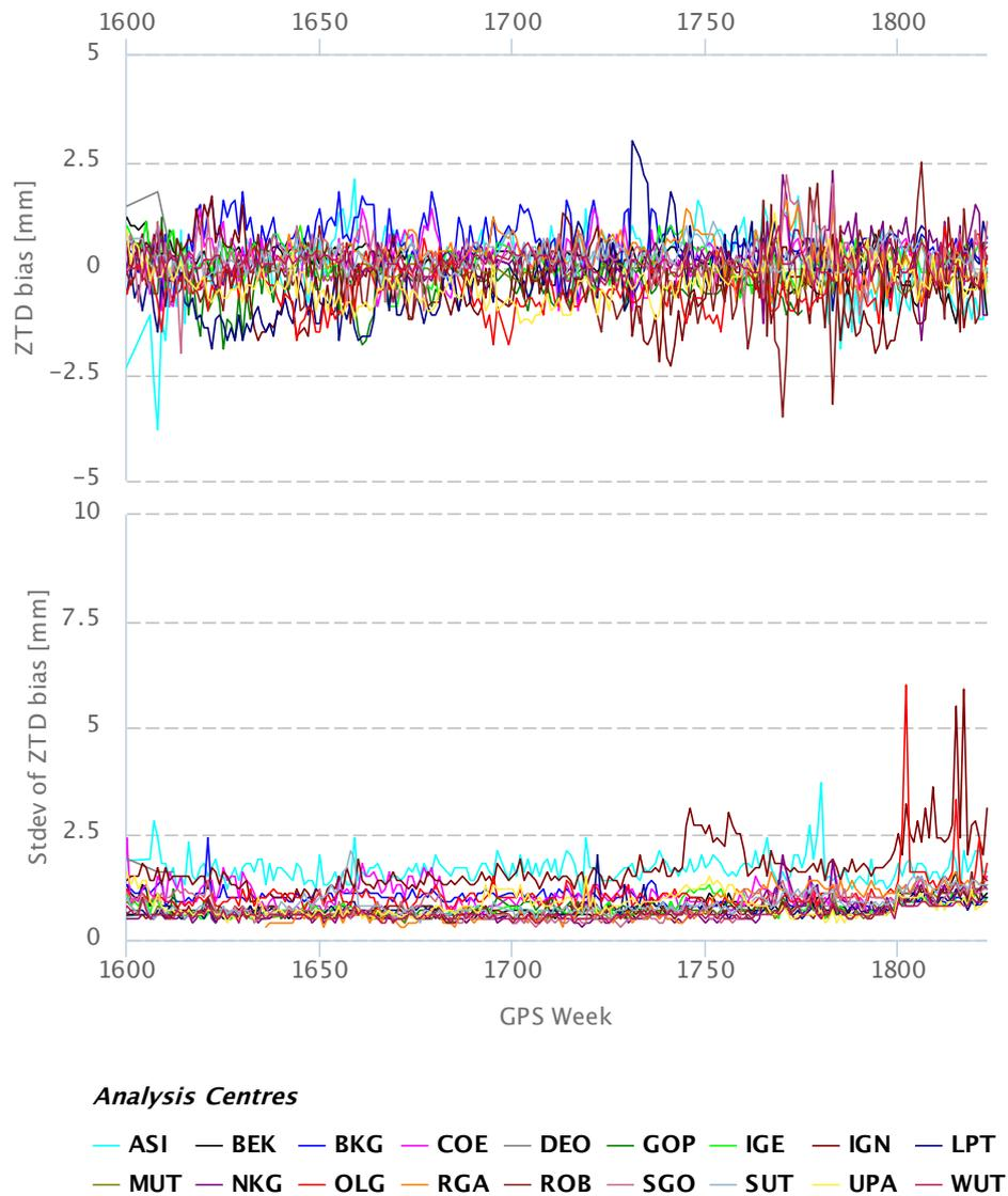
**Figure 6:** Weekly mean biases of LACs individual ZTD contributions with respect to the combined ZTD solution (mm ZTD); results from last 4 years of routine operation (Top). Standard deviation of weekly mean biases of LACs individual ZTD contributions with respect to the combined ZTD solution (mm ZTD); results from last 4 years of routine operation (Bottom).
