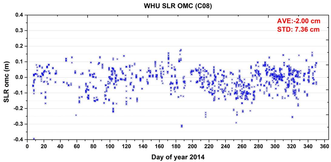
Figure 5: Beidou C08 orbit validation by SLR.
