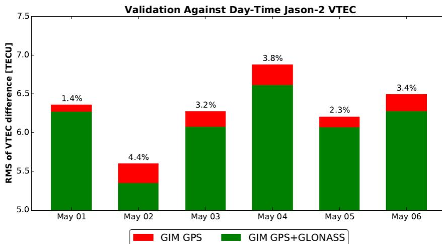
**Figure 6:** Day-time root mean square (RMS) of the difference between measured Jason-2 VTEC and JPL GIM VTEC derived from GPS alone (red) and combined GPS and GLONASS data (green). Each bar annotation indicates the daily improvement in the day-time VTEC difference RMS. Note the consistent and often significant improvement of the GPS and GLONASS GIM VTEC compared to that measured by an independent source.
