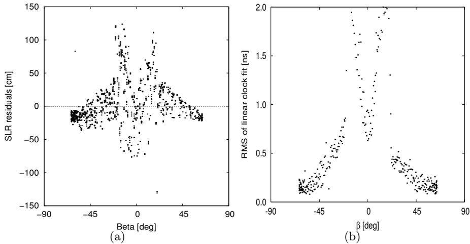
**Figure 4:** SLR residuals (a) and RMS of daily linear fit through estimated epoch-wise satellite clocks (b) of QZS-1 as a function of the elevation angle of the Sun over the satellite’s orbital plane (beta). The impact on orbit and clock estimates from ignoring the switch of QZSS’s attitude steering mode at beta angles of  $\pm 20$  degrees (Inaba et al. 2009) is clearly visible.
