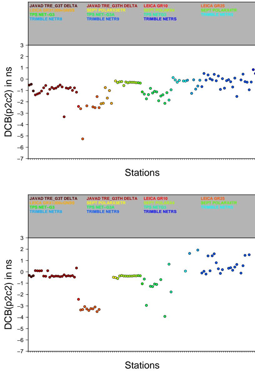
**Figure 6:** Monthly set of P2-C2 differential code biases for the GPS (top) and GLONASS (bottom) receiver components, for December 2014, computed at CODE.
