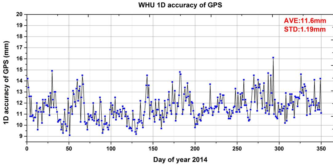
Figure 3: GPS orbit compared with IGS final solution.
