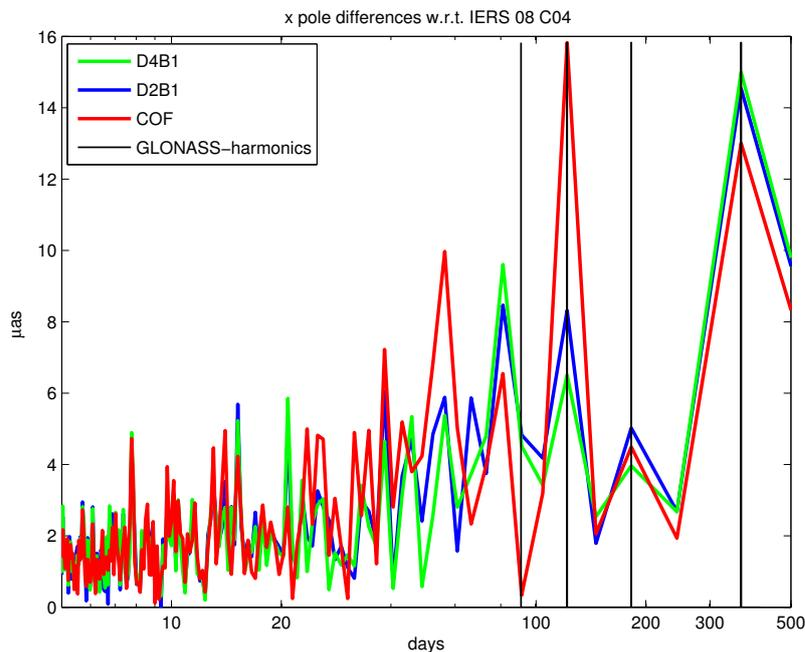
**Figure 3:** Amplitude spectra of differences of the polar motion coordinate  $x$  w.r.t. IERS 08 C04 for solutions obtained using the old ECOM (COF) and the extended ECOM with periodic  $D$ -terms up to 2pr (D2B1) and 4pr (D4B1). The spurious amplitude at 120 days is significantly reduced by the new ECOM.
