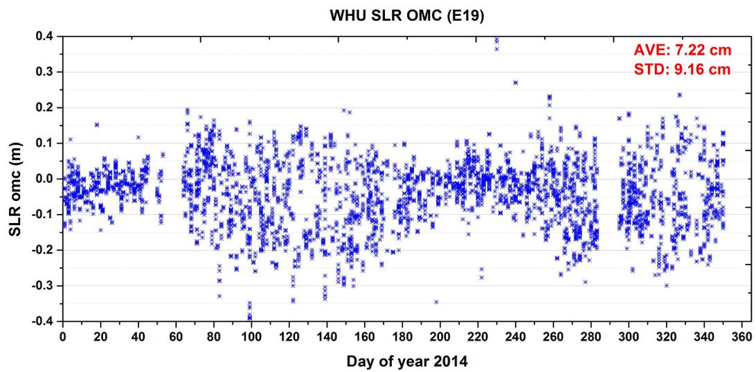
Figure 8: Galileo E19 orbit validation by SLR.
