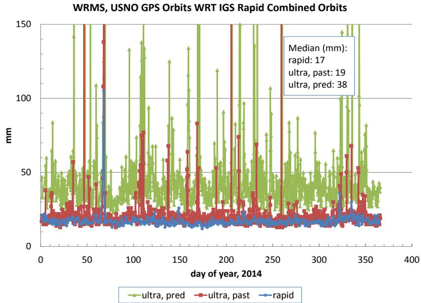
**Figure 1:** Weighted RMS of USNO GPS orbit estimates with respect to IGS Rapid Combination, 2014. “Ultra, past” refers to 24-hour post-processed section of USNO ultra-rapid orbits. “Ultra, pred” refers to first six hours of ultra-rapid orbit prediction.
