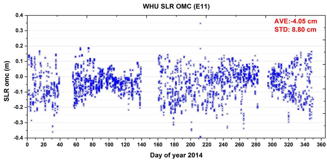
Figure 7: Galileo E11 orbit validation by SLR.
