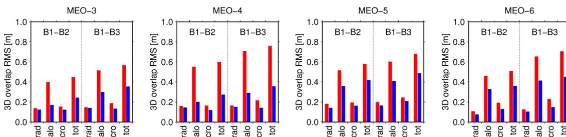
**Figure 3:** Day-to-day orbit overlap differences (RMS) computed for each MEO spacecraft over a five-month processing period. The standard PCO-only solution is shown in red, the advanced PCV-based solution in blue
