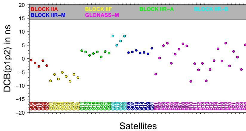
**Figure 2:** Monthly set of P1–P2 differential code biases for the GPS and GLONASS constellation, for December 2014, computed at CODE.
