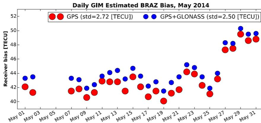
**Figure 5:** JPL GIM bias time-series for station BRAZ derived for GPS data alone (GPS) and combined GPS and GLONASS data (GPS+GLONASS) for May, 2014. Data were not available for May 3–6. Note the decreased station bias standard deviation (std) in the GPS+GLONASS result.
