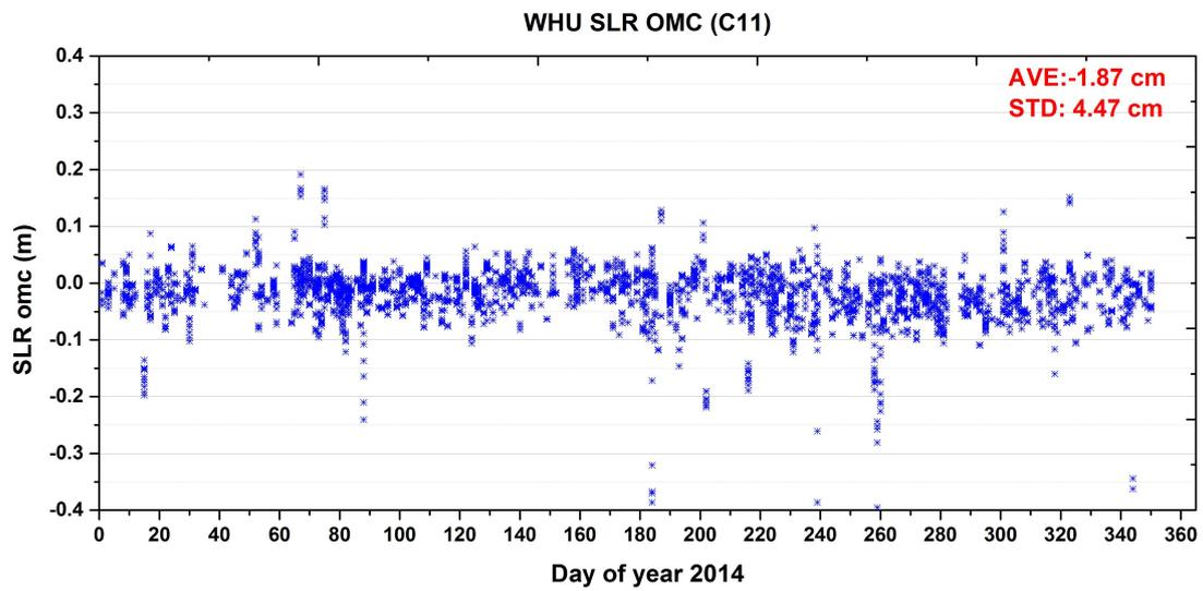
Figure 6: Beidou C11 orbit validation by SLR.
