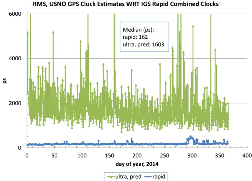
**Figure 2:** RMS of USNO GPS rapid clock estimates and ultra-rapid clock predictions with respect to IGS Rapid Combination, 2014.
