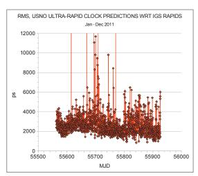
**Figure 2:** RMS/standard deviation of USNO rapid GPS clock estimates (left) and RMS of USNO ultra-rapid GPS clock predictions (right) with respect to IGS Rapid Combination, 2011.
