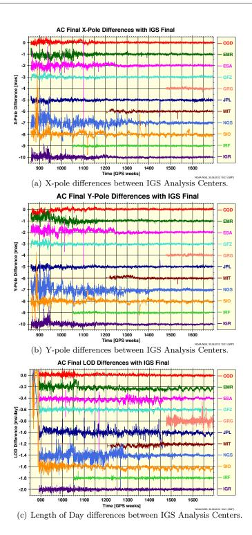
**Figure 2:** Comparison of the IGS final products with the AC contributions for the Earth rotation parameters.
