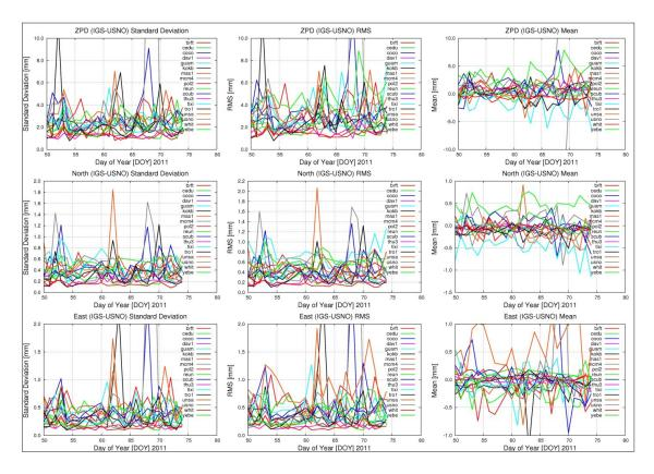
**Figure 1:** Comparison of USNO test troposphere solutions to existing IGS Final Troposphere estimates, in preparation for operational transition to USNO. ZPD = total zenith troposphere delay. Days of year 50–74 (28 Feb—14 Mar) 2011. From Byram at al. (2011).
