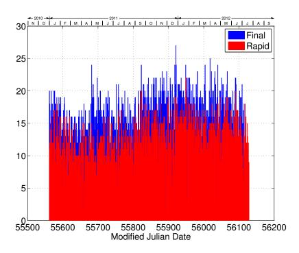
**Figure 6:** Histogram of the daily number of clocks in the IGS Final and Rapid timescale filters having phase estimate stabilities better than  $3 \cdot 10^{-15}$  at  $\tau = 21,600\,\mathrm{s}$  as measured by the Hadamard deviation statistic.
