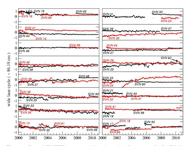
**Figure 4:** Observed GPS WSB between year 2000 and year 2010. One curve per Satellite Vehicle Number (SVN) is shown.
