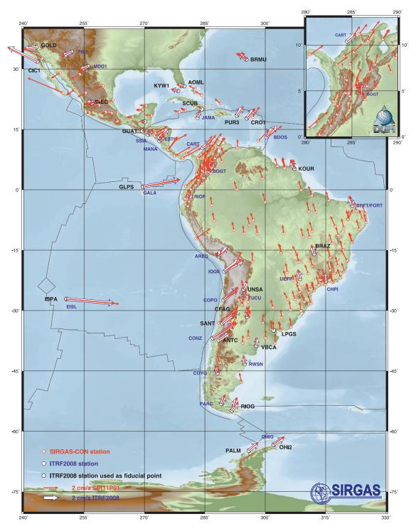
Figure 3: Horizontal velocities of the multi-year solution SIR11P01.
