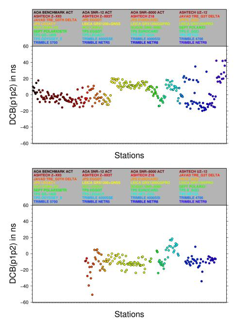
**Figure 3:** Monthly set of P1-P2 differential code biases for the GPS (top) and GLONASS (bottom) receiver components, for December 2011, computed at CODE.
