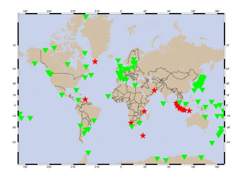
**Figure 1:** Current TIGA Network. Only stations are accepted as TIGA where, tide gauge, GNSS and leveling data is made public. (green triangles: TIGA Observing Stations, red stars: pending station approval)
