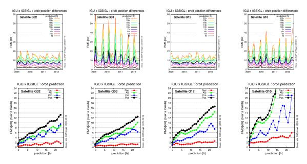
Figure 3: Plots show time—series of GPS satellite orbit quality (top) and the prediction of radial, along—track and cross—track monthly dependence on prediction (bottom). Two left plots show non—eclipsing and right eclipsing satellites. G02 and G12 are Block IIR, while G03 and G10 Block IIA satellites. Colors shows accuracy for fitted (0h) and predicted positions (1h, 4h, 7h, 10h, 13h, 16h, 19h, 22h) The orbits are comparedo to IGS finals
