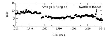
**Figure 3:** Global RMS residuals (up component) between our weekly network solution and the IGS weekly combined solution. From February 22, 2009 (GPS week 1520) to June 6, 2011 (GPS week 1640).
