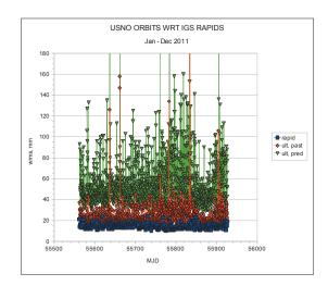
**Figure 1:** Weighted RMS of USNO GPS orbit estimates with respect to IGS Rapid Combination, 2011. "Ult, past" refers to 24–hour post–processed section of USNO ultra–rapid orbits. "Ult, pred" refers to first six hours of ultra–rapid orbit prediction.
