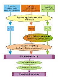
Figure 4: Flowchart of the TIGA combination implemented at AIUB.
