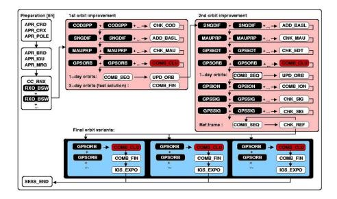
Figure 1: GOP processing scheme based on 6-hour data batch and long-arc combination
