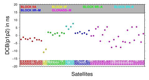
Figure 2: Monthly set of P1-P2 differential code biases for the GPS and GLONASS constellation, for December 2011, computed at CODE.
