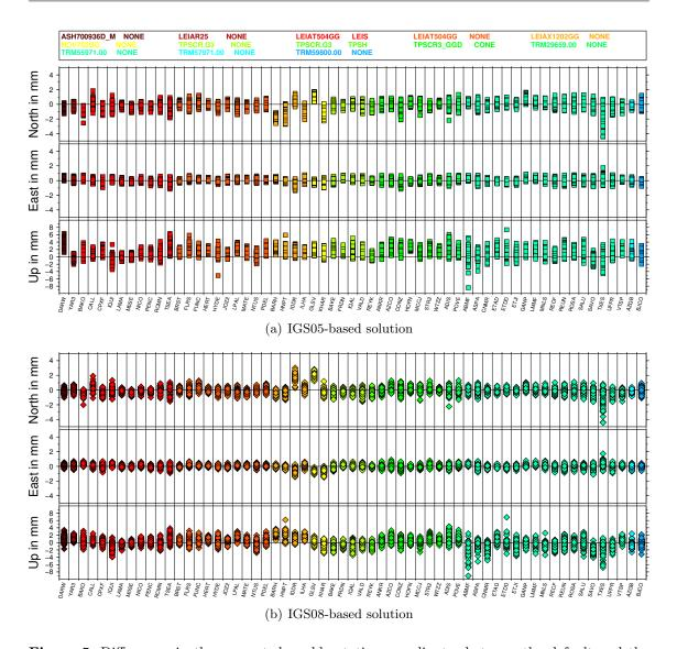
**Figure 5:** Differences in the computed weekly station coordinates between the default and the solution with the GPS/GLONASS bias estimation.
