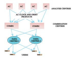
Figure 3: RTS GNSS product distribution architecture.
