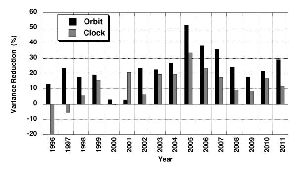
Figure 1: Variance reduction in orbit and clock precision of JPL's first IGS08-based reanalysis of historical GPS data relative to our IGS05-based reanalysis. Precision is measured through the root-mean-square (RMS) of differences between neighboring daily 30-hour solutions during the overlapping 6-hour period. The average orbit and clock variance reduction for 1996-2011 is 25% and 12%, respectively.
