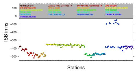
**Figure 9:** GLONASS-GPS intersystem clock/time biases/differences as computed for a set of IGS stations, for 12 January 2012.
